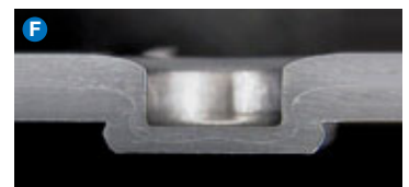
Aluminium 1.5 mm Aluminium 1.5 mm
