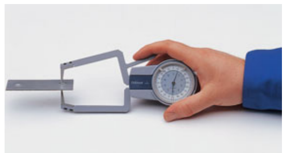
Testing the residual material thickness ST
